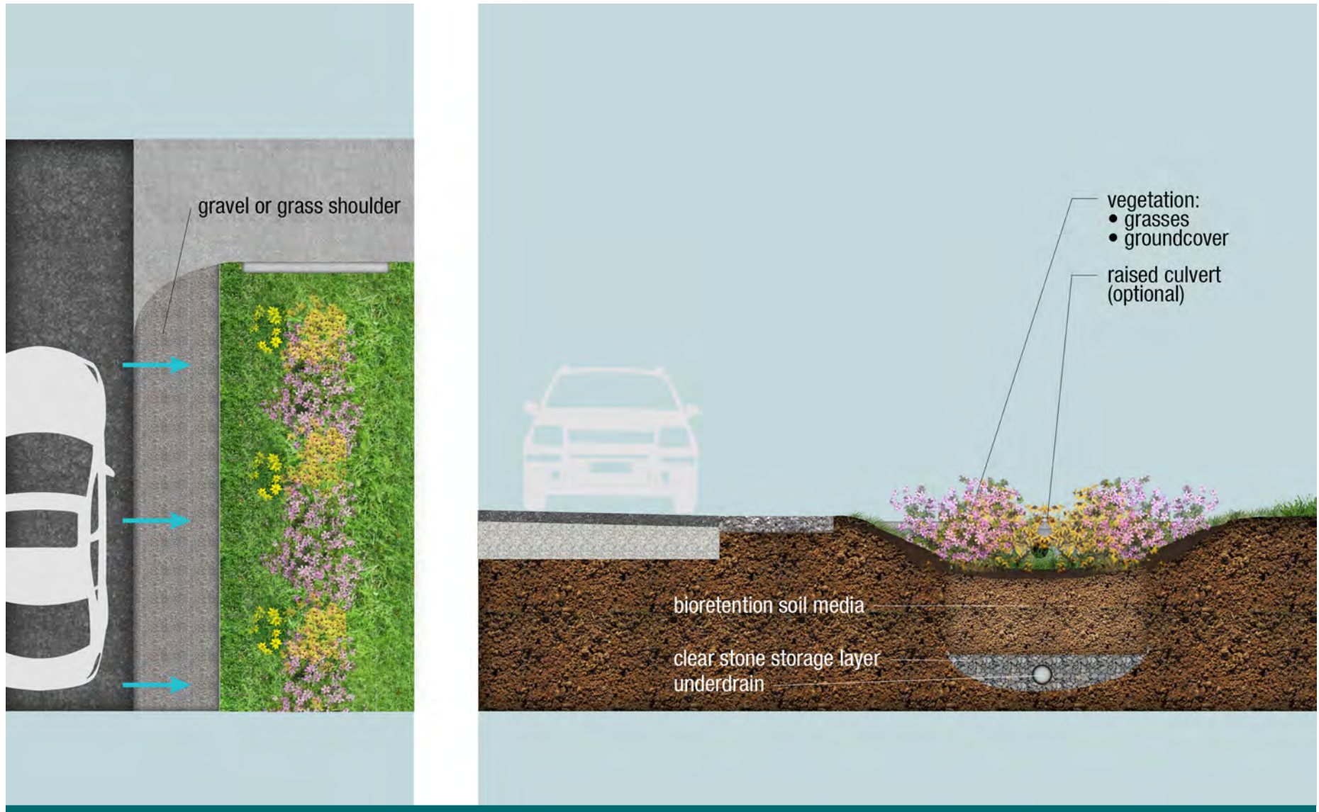
Figure 2.2.5: Bioswale plan view [left] and cross-section [right]
