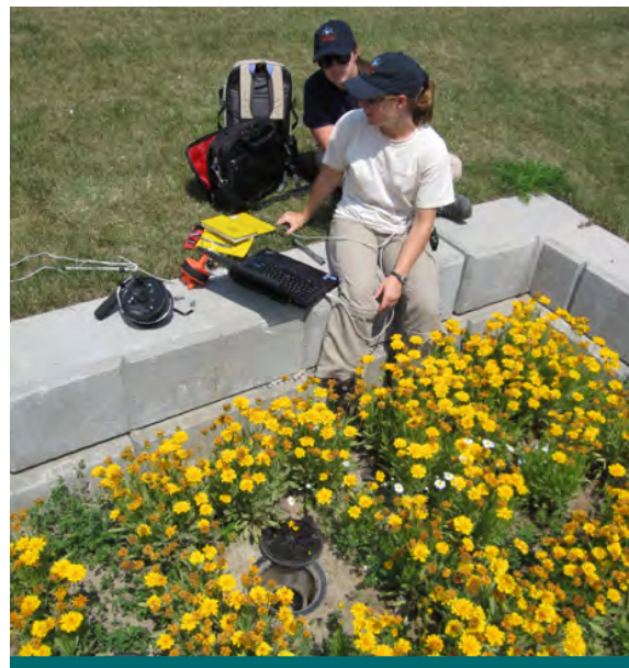
Figure 9.6.2: The water level logger has been pulled out of the bioretention cell observation well. The water level data from the logger is being downloaded directly to a laptop before being put back in the well. (Source: CVC)
