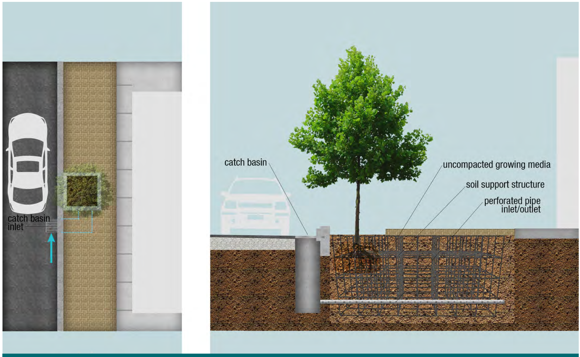
Figure 2.4.5: Soil support system plan view [left] and cross-section [right]
